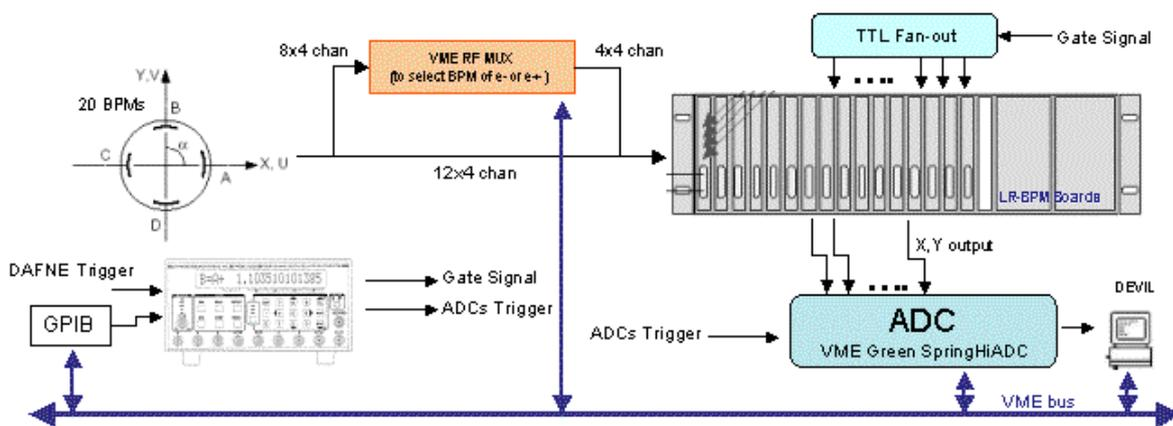
Figure 5: Block diagram of the trajectory acquisition system.
