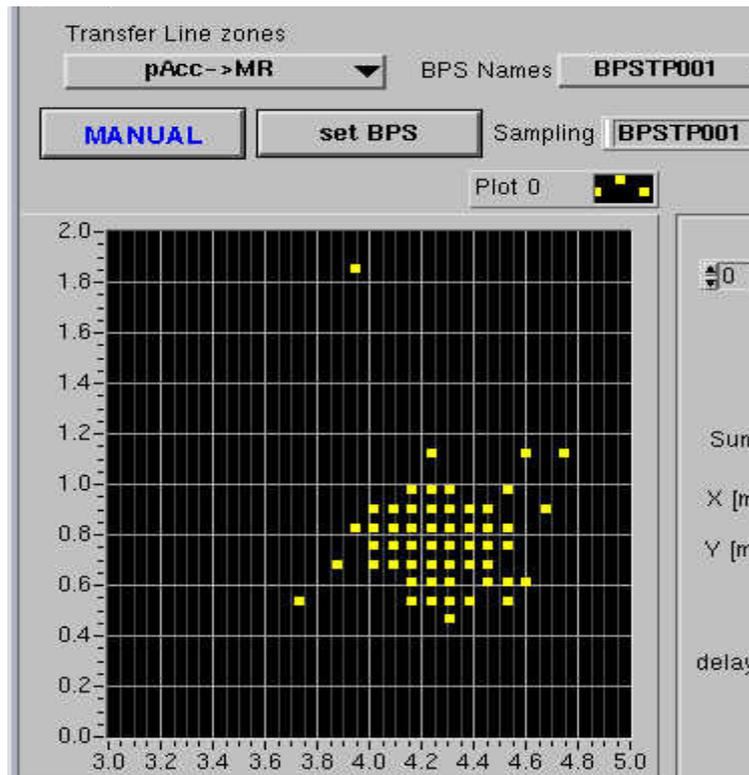
Figure 7a: Data acquisition at different beam passages for BPSTP001 (axis scale in  $\sigma_x \sim 0.20$  mm,  $\sigma_y \sim 0.20$  mm @ DR current  $I = 25$  mA).
