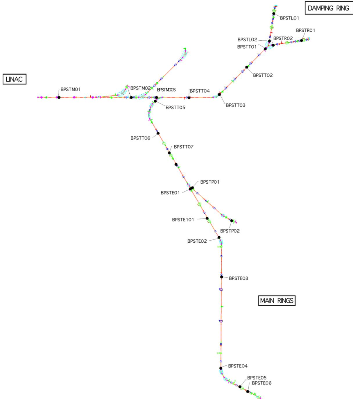
Figure 1: BPMs along the Transfer Line.
