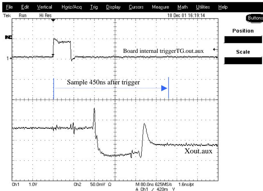
Figure 6: Typical Log board output signals
