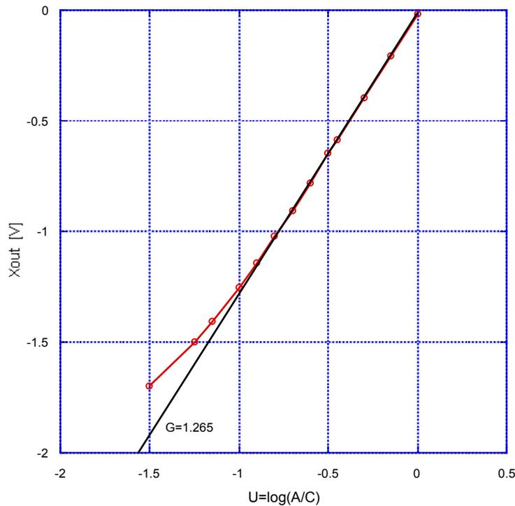
Figure 3: LR-BPM board gain.
