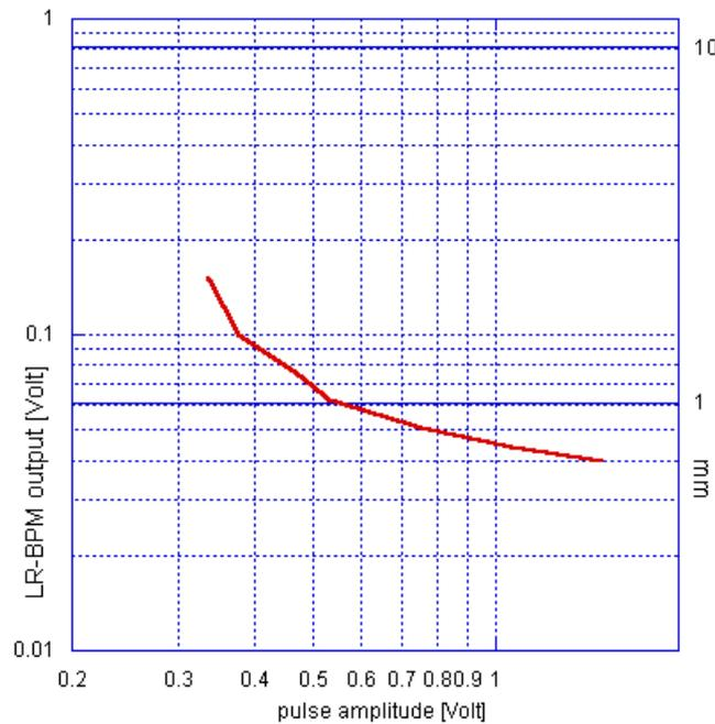
Figure 4: Noise error vs pulse amplitude.
