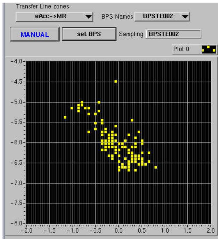
Figure 7b: Data acquisition at different beam passages for BPSTPE002 (axis scale in  $\sigma_x \sim 0.25$  mm,  $\sigma_y \sim 0.25$  mm @ DR current  $I = 20$  mA).
