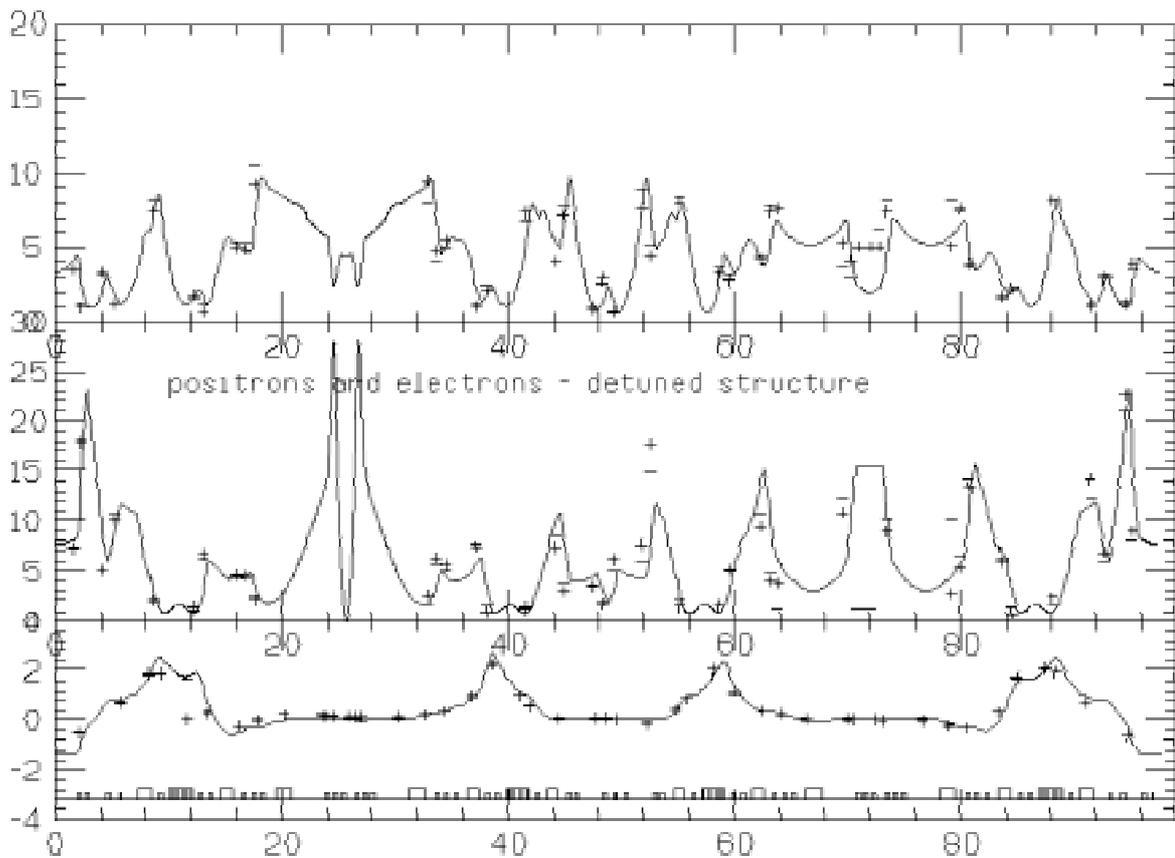
Figure 1 – Measured betatron functions and dispersion on positron (+) and electron ring (-).
