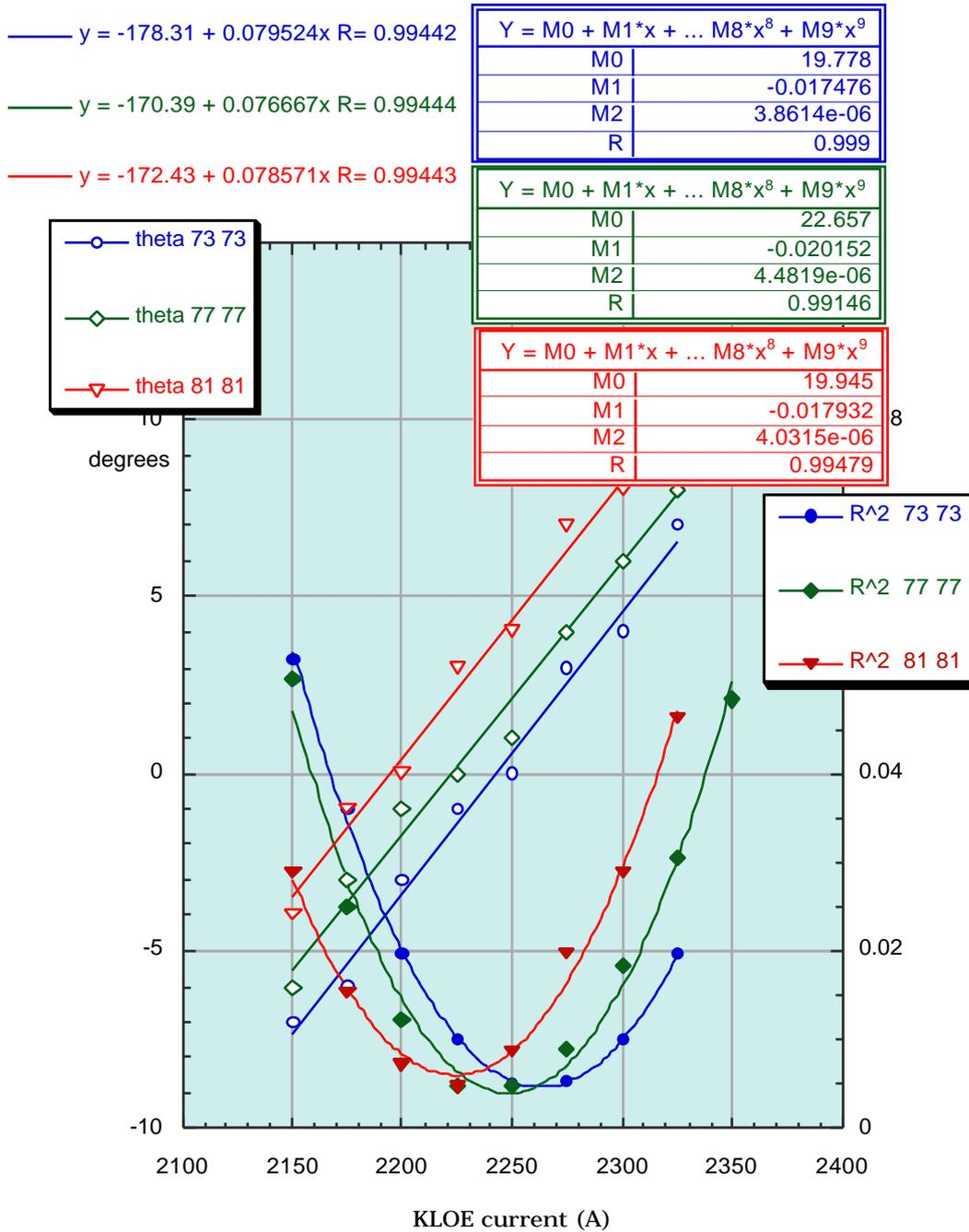
Figure 4 – Coupling and orientation at the SLM as a function of KLOE field with  $C_1 = -C_2$  at different currents on positron ring
