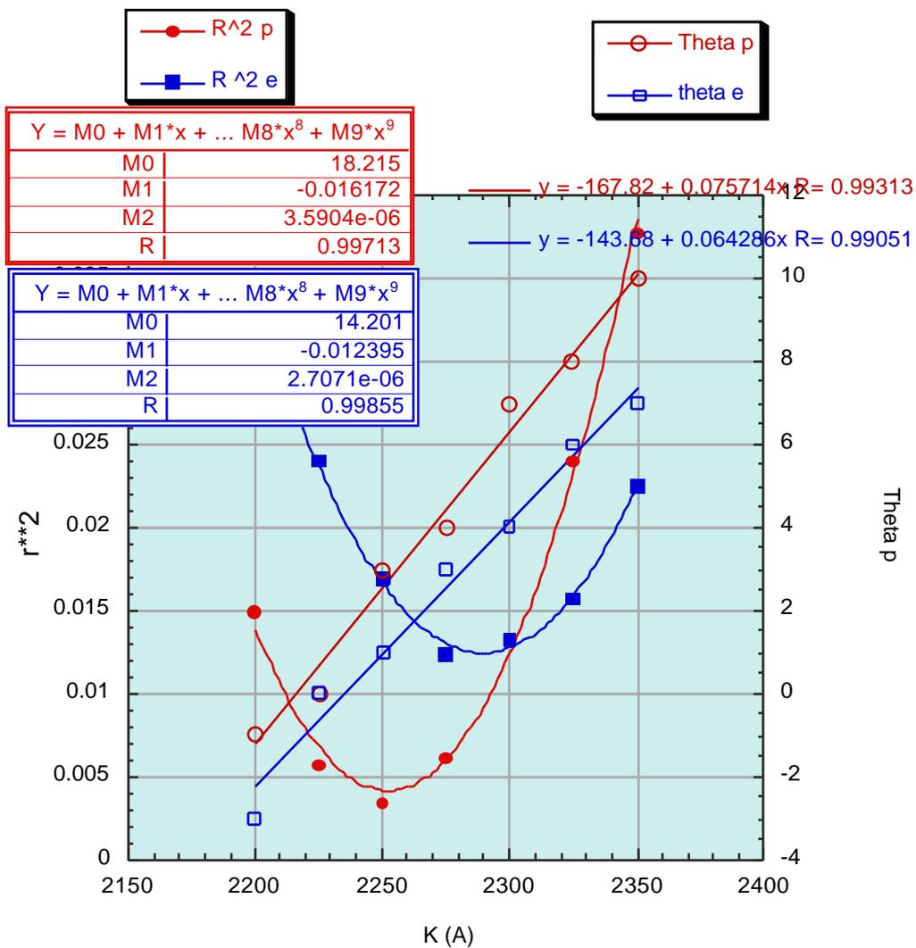
Figure 3 – Coupling and orientation at the SLM as a function of KLOE field with  $C_1 = -77$  and  $C_2 = 77A$
