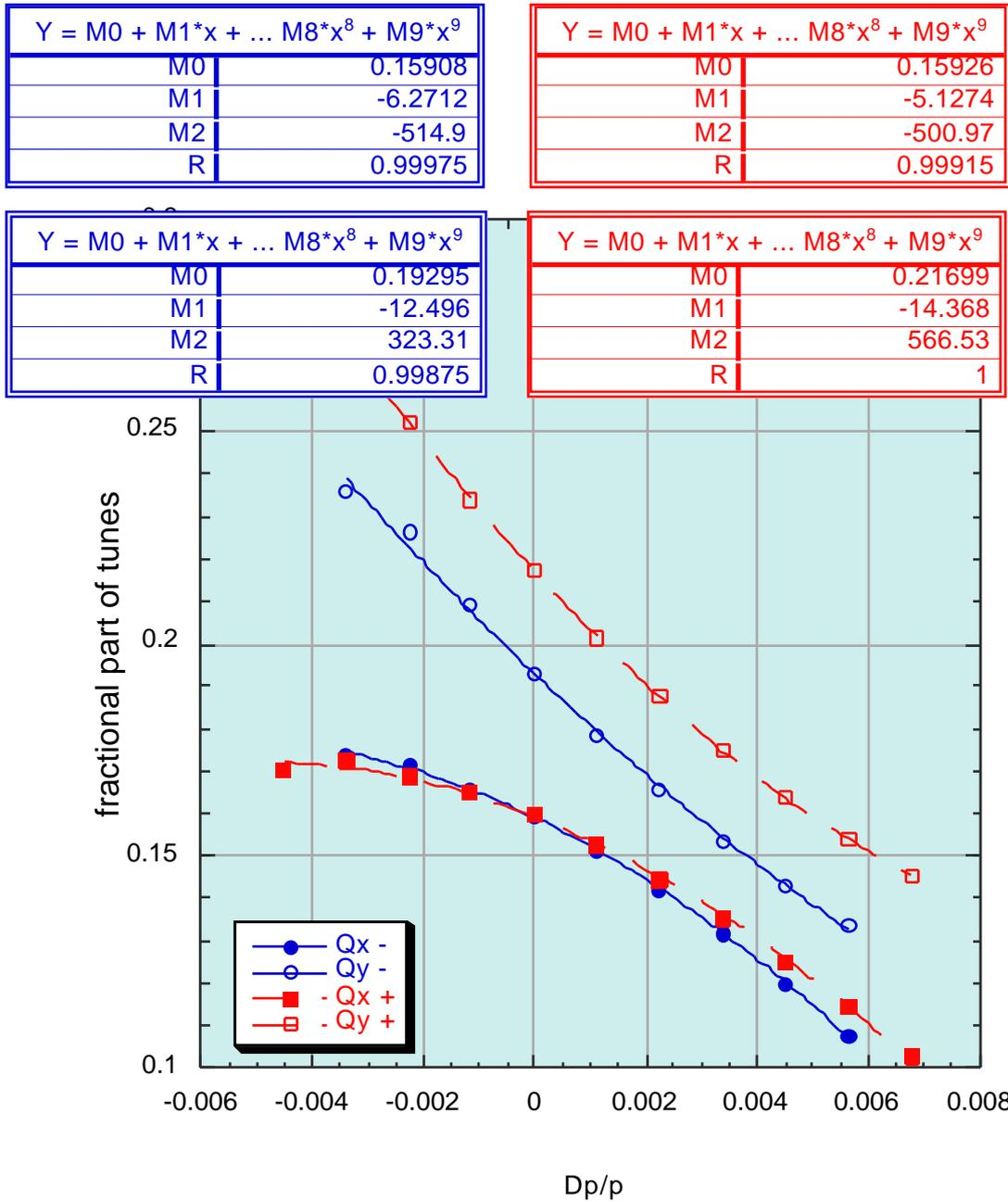
Figure 2 – Tunes vs. energy variation with sextupoles off in electron (left equations, full lines) and positron (right equations, dashed lines) rings.
