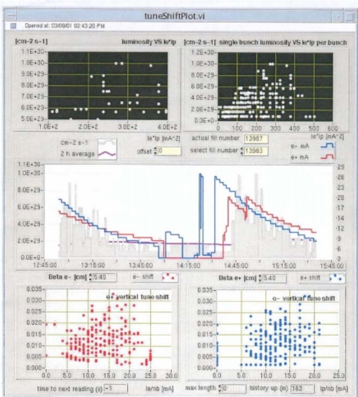
Figure 7 – Second day of collisions reaching luminosity of  $10^{30} \text{ cm}^2 \text{ sec}^{-1}$
