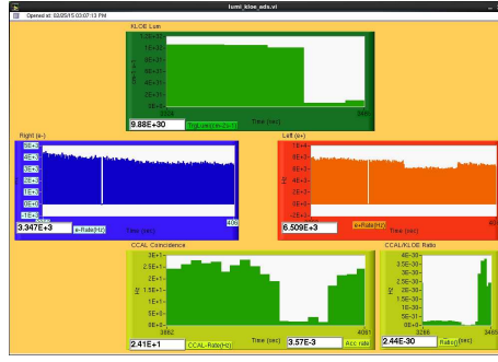
Figure 5: Screen-shot of the DAΦNE control system application performing data acquisition of the CCALT luminometer test set-up. In the center bottom panel is presented the effect on the coincidence rate obtained moving the two beams out of collisions.
