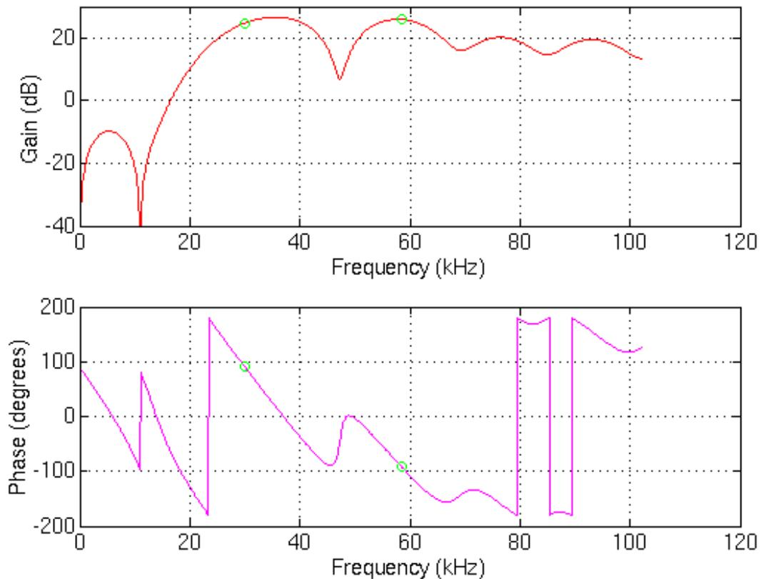
**FIGURE 3.** Dual-peak filter response with a notch at the mode zero frequency
