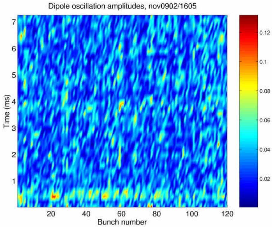
FIGURE 4. Bunch oscillation amplitudes filtered around synchrotron frequency
