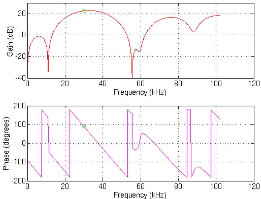
**FIGURE 2.** Frequency response of the quadrupole open-loop filter with a peak at 30 kHz and a quadrupole notch at 56 kHz.
