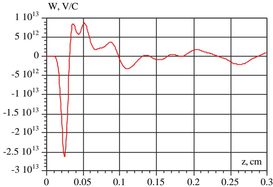
Fig. 4 - Accumulator ring wake potential for 5 mm Gaussian bunch.
