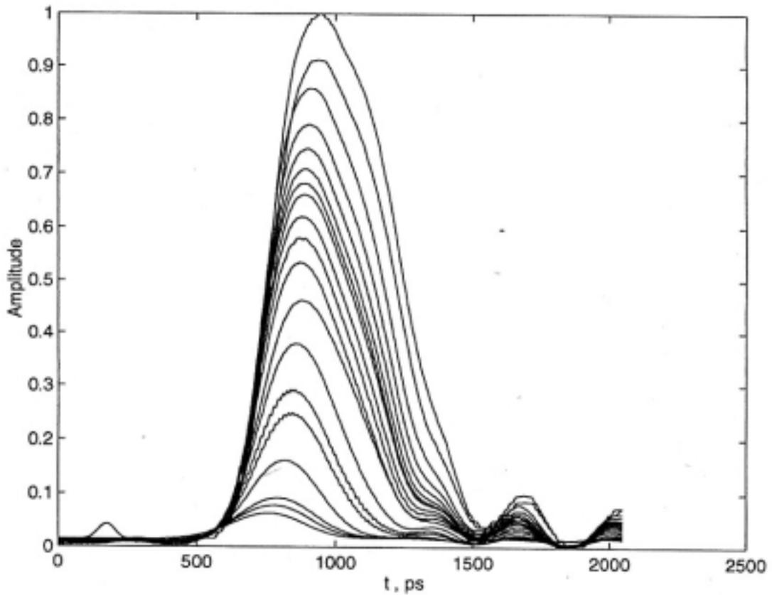
Fig. 8 - Bunch shape for different average bunch currents
