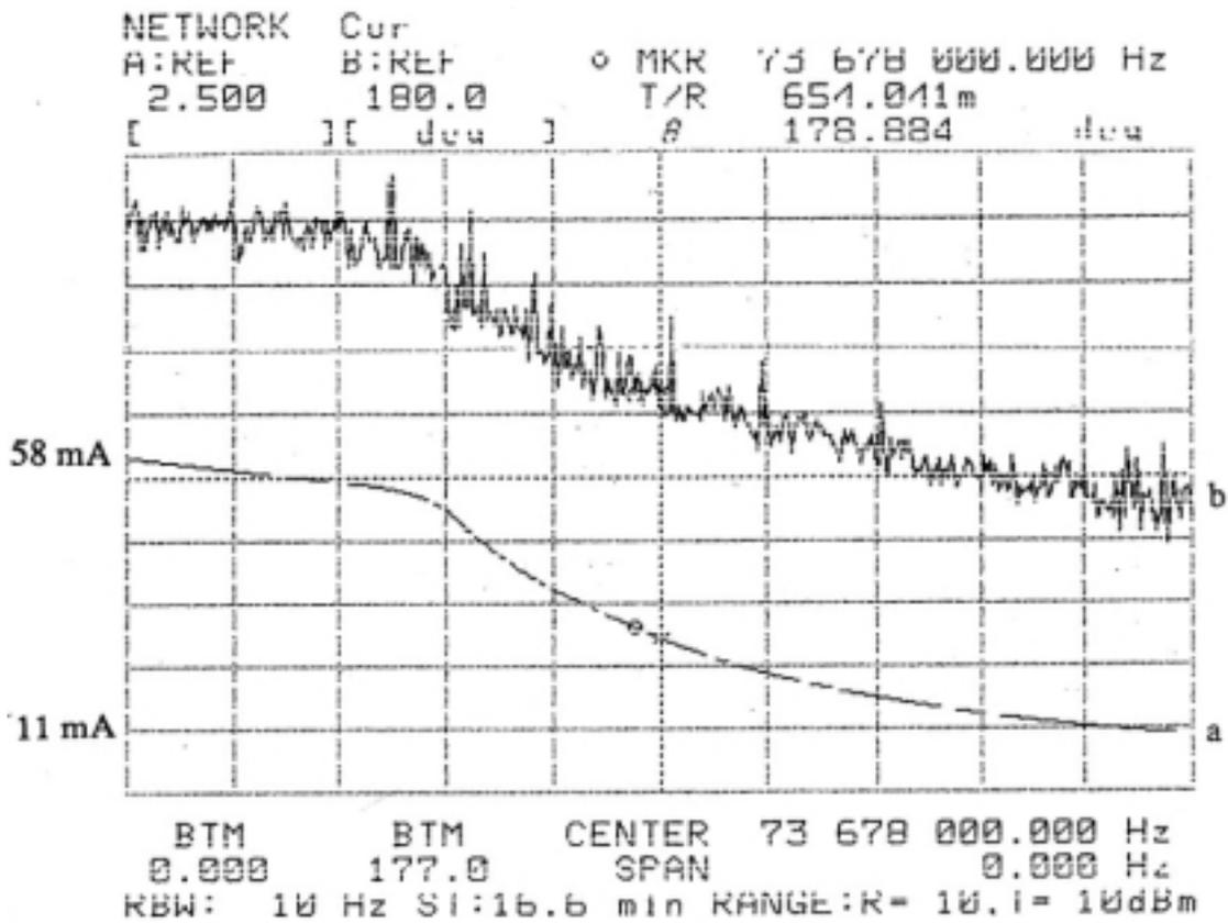
Fig. 2 - Measured average bunch current (a) and relative synchronous phase shift (b) at  $\hat{V}_{rf} = 60$  kV.
