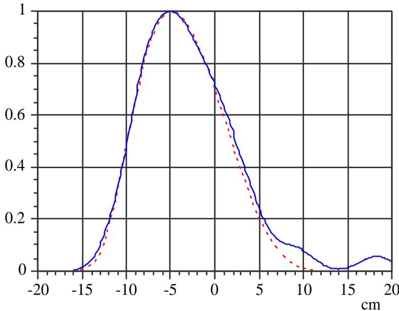
Fig. 9- Bunch shape at  $I = 28$  mA: solid line - measurement; dotted line - fit with  $Z(\omega) = (600 + j6.2e - 08\omega)\Omega$
