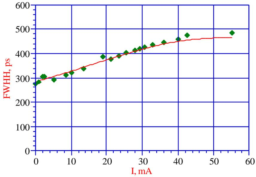
Fig. 7 - Bunch lengthening in the accumulator ring (full width at half maximum): dots - measurement results; solid line - numerical simulation.
