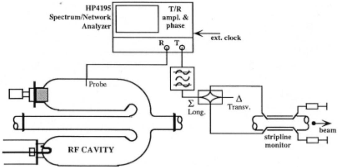
Fig. 1 - Block diagram of phase shift measurement set.
