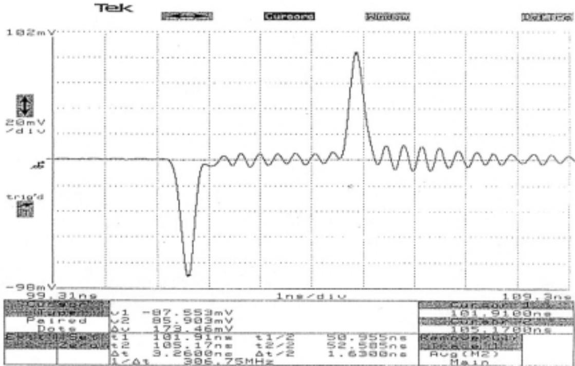
Fig. 5 - Typical stripline response at low-current. The small superimposed oscillation occurs at the first TM waveguide mode in the round beam pipe ( $\Phi \sim 86$  mm).
