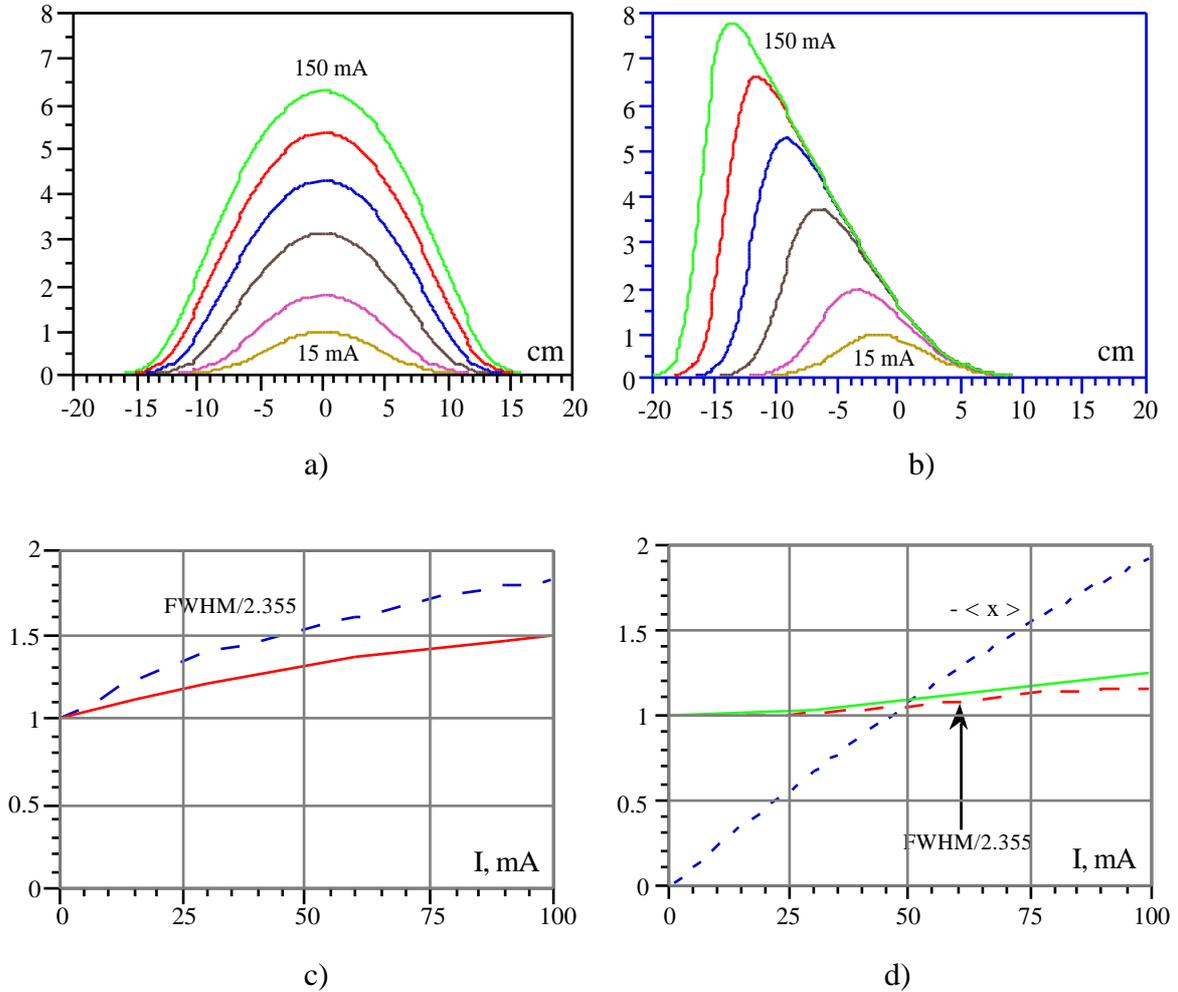
Fig. 3 - Examples of bunch shape and relative bunch lengthening for purely inductive (a, c) and purely resistive (b, d) impedance: solid line - rms bunch length; long-dashed line - full width at half maximum; short-dashed line - shift of bunch center of mass.
