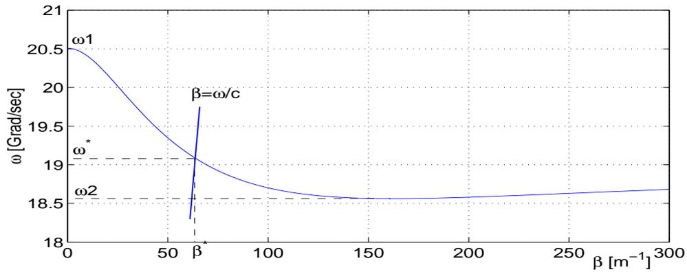
Figure 1: dispersion curve of the RF separator EH<sub>11</sub> mode
