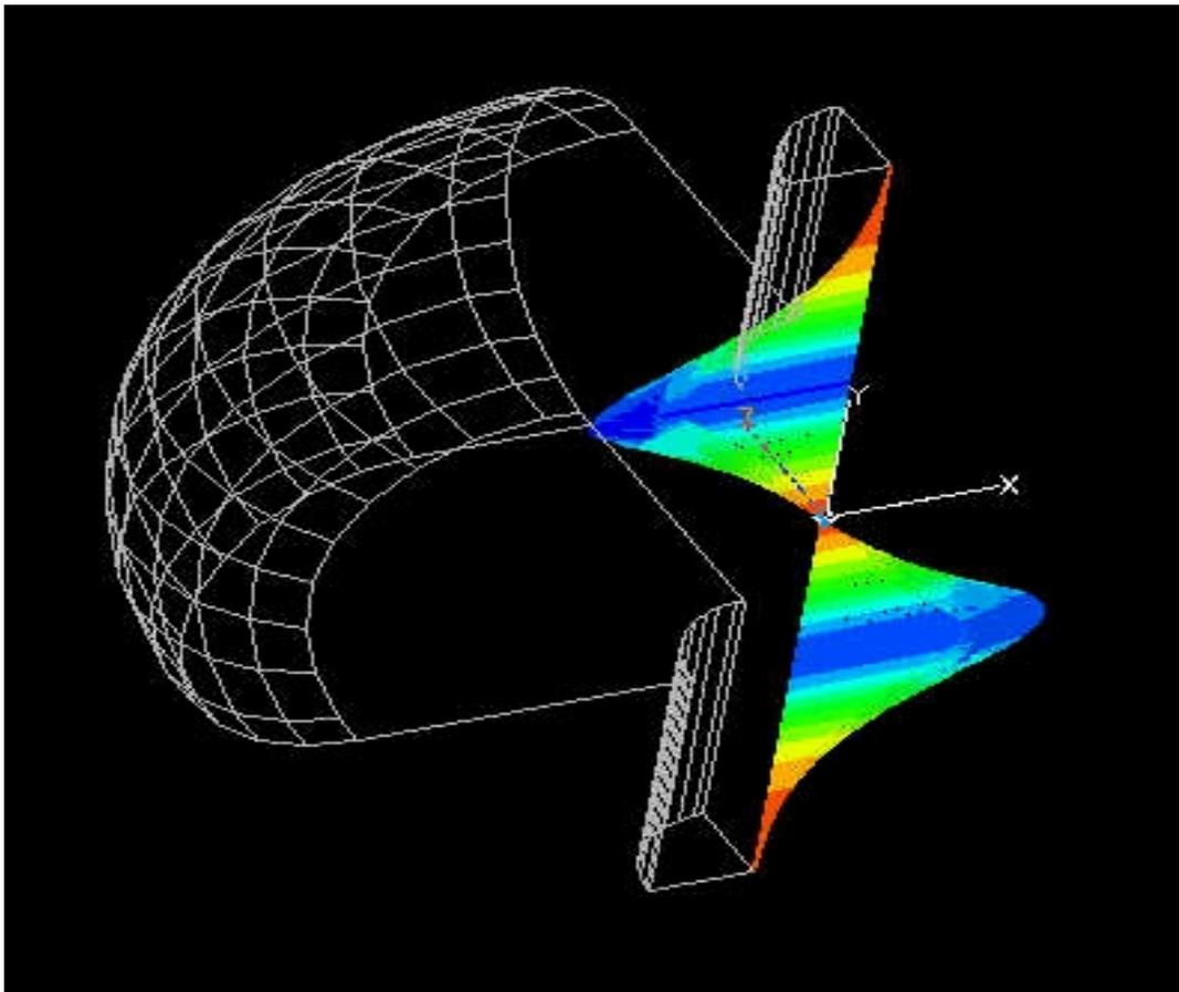
Figure 10: HFSS model of a SW single-cell cavity
