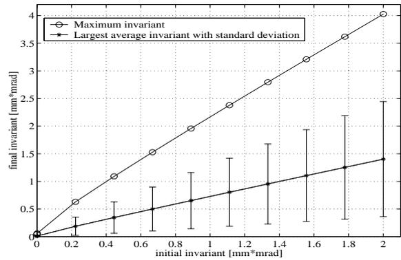
Figure 8:  $\hat{I}_{o\_max}$  and  $\hat{I}_{o\_ave}$  as function of the injection Courant-Snyder invariant
