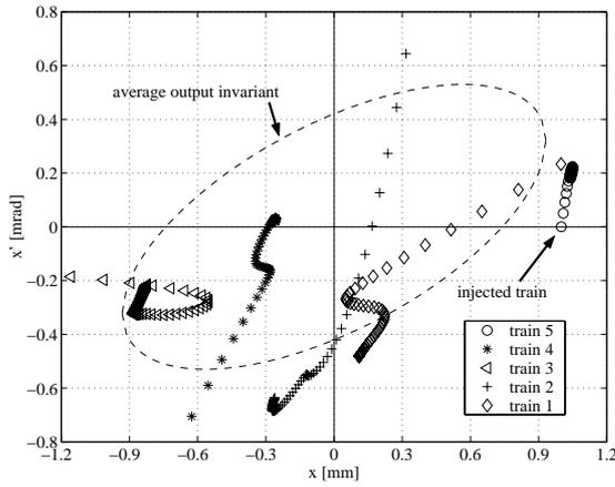
Figure 6a: bunch train phase space footprint for an injection offset of 1 mm
