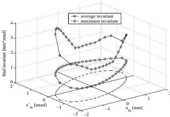
Figure 7:  $I_{o\_max}$  and  $I_{o\_ave}$  for a given  $I_{in}$  for various betatron phases
